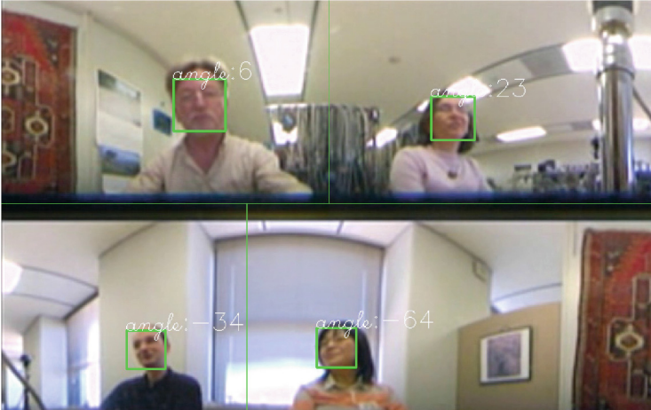
Fig. 2. Screenshot of TableTalk with face detection and head yaw angle
